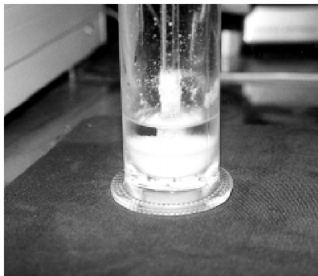
Fig. 2: Precipitation of white crystals, reaction time 1.5 h
